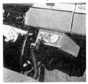
About the only trouble you're likely to face is having bounces and jolts jiggle the handset turning S1 on and off and cutting the speaker in and out. Should this happen, simply adjust the hanger tension so the handset is pressed firmly against the control box.
