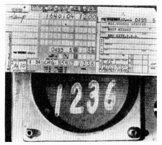
An oscilloscope displays four numbers scanned by an experimental IBM optical reader from a store sales slip. IBM is seeking new ways to apply advanced handling techniques in the retail industry by eliminating punched cards.
