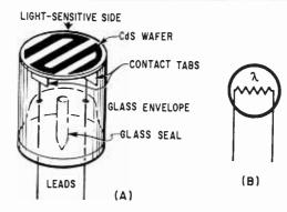
Fig. 4. Construction of a typical cadmium sulphide photoconductor (A) and symbol (B).
