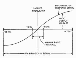
Comparison of the FM broadcast and narrowband communications FM transmitted signals.
