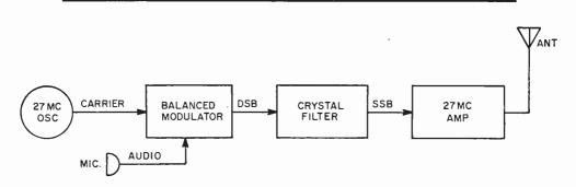
Fig. 6. Block diagram of a simplified SSB CB transmitter. Early stages provide same functions described in Fig. 5. The DSB signal, however, is applied to crystal filter for removing of one sideband. Then SSB signal is amplified.
