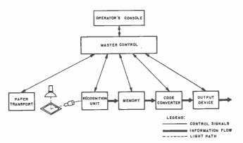
An overall view (above) of Philco's new General Purpose Print Reader system. Block diagram (left) shows signal flows in the system that reads a printed page.
