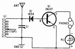
Fig. 8. Sun bathers will enjoy making and using the solar-powered AM receiver diagrammed above. PC replaces 1.5-volt dry cell.
