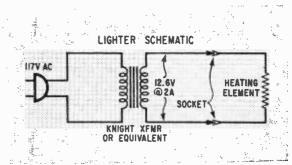
Switch, fuse, and indicator can be added.
