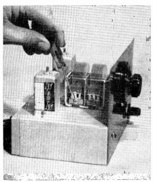
It is important that the BCB Booster be aligned carefully so that it tracks accurately. Trimmer capacitor screws (one of two pointed out by screw-driver) are used to align the RF preamplifier to signals on the high end of the BC band.
