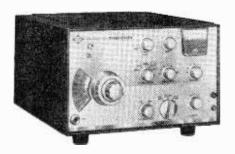
circuitry. The transmitter section delivers a full 300 watts P.E.P., using modern shift carrier, with a choice of both upper and lower sidebands. Full 500-kc. coverage on 80, 40, and 20 meters. The Galaxy and matching accessories are now available at all leading ham distributors for \$349.95. (Complete specifications are yours for the asking. Galaxy Industries, 10 South 34th Street, Council Bluffs, Iowa.)
