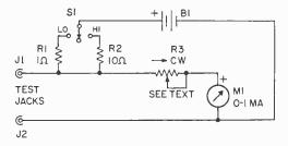
Close examination of circuit reveals that external resistor serves as the meter shunt.
