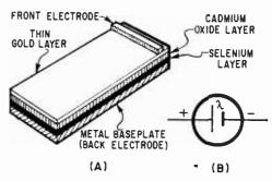
Fig. 5. Cross-section view of a selenium photovoltaic cell (A) and its symbol (B).
