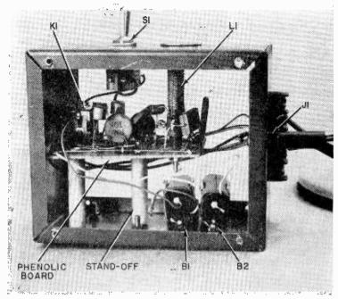
Inside view of the ProxSwitch with top and bottom covers off. Almost all of the parts are mounted on a prefab phenolic board.
