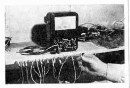
CLIP LEADS to a piece of wire strung between screws or nails to keep them handy.
