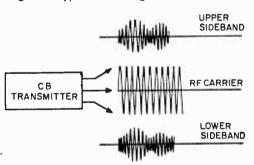
Fig. 2. Actual CB stgnal. Audio appears only in two sidebands, carrier is steady.
