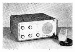
Mark Products Sidewinder SSB-27 was the first single-sideband rig to appear on the CB market. Its RF carrier is reduced to less than one-thousandths that of a normal CB carrier. Likewise, one sideband is suppressed to one ten-thousandths that of usual sideband power. Remaining sideband receives nearly all output wattage. Selector switch on front panel enables operator to transmit on upper or lower sideband on any of five channels. Priced at \$299.50.
