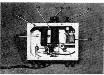
Under chassis view of the booster showing part placement. Note that power transformer T3 is mounted on a side flange. Filter capacitors C5 and C6 are mounted to terminal strips.
