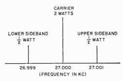
Fig. 4. Graph of how output power is divided among three parts of CB signal. Carrier receives twice as much as its two sidebands.
