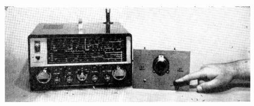
Separating "wheat from the chaf" is the job of this tunable broadcast-band preamp that connects to any receiver
