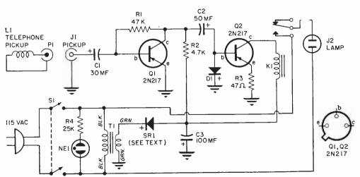
A close look reveals that the transistor circuit is line isolated by transformer T1.
