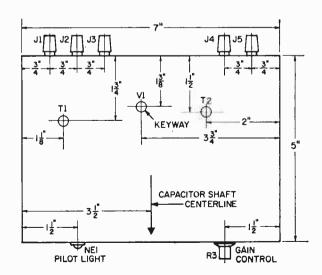
Top view drawing showing parts placement on the BCB Booster's chassis. Rubber cement white paper to the top, front and back sides of the chassis and mark all hole centers as shown in the drawing. Mounting holes for the tuning capacitor are marked with the unit held in place and its shaft located along the centerline. Parts mounted on the front and back sides are located midway from top to bottom of chassis.
