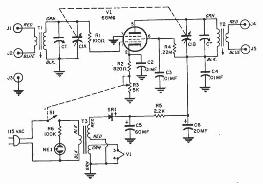
Schematic diagram for the BCB Booster. Although the circuit may seem uncomplicated, considerable design and model-making effort was expended to insure maximum gain over the tuning range without oscillations.
