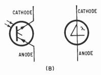
Fig. 6. Cross-section view of a GE silicon light activated switch (A) made by General Electric, and two schematic symbols (B) currently used by electronic engineers.
