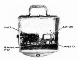
Inside view of lunch box portable prior to installation of loudspeaker and wood panel.
