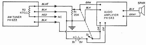
Interconnection diagram for the lunch box portable. AM tuner and audio amplifier are purchased, prewired units with color-coded leads. Interconnect these units after all parts except speaker have been mounted.
