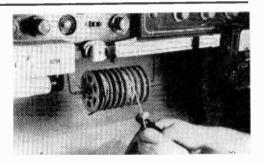
reel shaft; the other end of each wire is mounted under a workbench shelf with wood screws. Shape the wire brackets so they can pivot on their mounting screws, allowing easy "swing-away" removal for adding, changing or refilling the reels. Different colored reels will help you pick out the wire you need at a glance.
