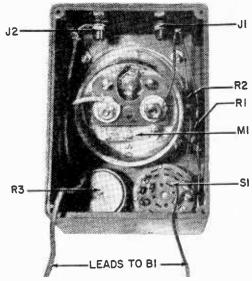
Bottum-up view of Lo-Ohmmeter shows parts placement—battery mounts on bottom cover.
