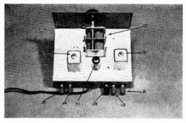
Compare the photo (left) against the detail topview drawing on page 78. Part placement is critical to insure satisfactory operation with no oscillations. If you wish, the BCB Booster can be installed in a cabinet.
