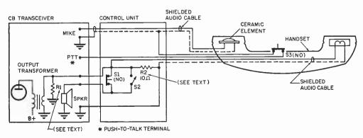
The schematic diagram reveals that no changes were made to the original microphone circuit; ear piece is nothing more than an extension speaker.
