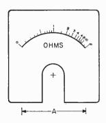
Meter scale drawing (above) and meter-swing vs. resistance graph (right) are used to calibrate any meter (see text).
