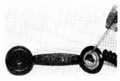
The surplus handset comes with a carbon mike that cannot be used. New mike is installed in mouth-piece surrounded by foam padding to prevent vibration pickup.
