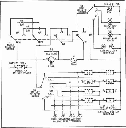
Be careful wiring the tester. Use colored leads to permit rapid wire tracing.
