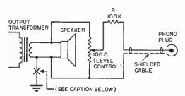
Diagram for adding a tape recorder pick-up jack to a radio or amplifier. Ground connection should be broken if hum occurs.
