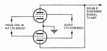
Fig. 5. Typical circuit for suppressing RF carrier. RF from oscillator is applied to grids in pushpull, plates are connected in parallel. This causes steady RF to buck itself out. Audio is supplied to screen grids in push-pull.
